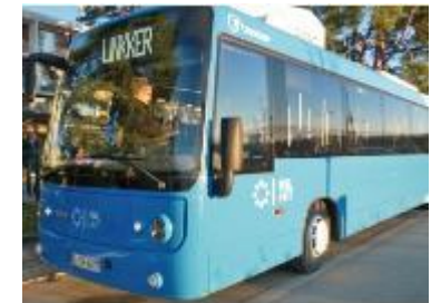
Fast-charging electric bus system
